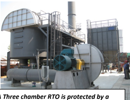
A Three chamber RTO is protected by a pulse jet dust collect is shown in the background.
